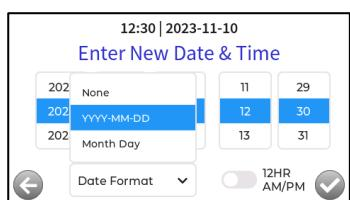
The Enter New Date & Time screen can be reached by selecting the “Date/Time” button. On this screen you may select the date and time by scrolling to the desired values. This screen also provides the option to toggle the date on/off or into different formats, and to toggle the 12HR AM/PM format off and display time in the 24HR format. There will also be a “Back” button to return to the Select Tool screen and a “Confirm” button to store the date and time you have chosen.
