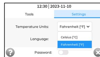
Pressing “Settings” will display drop-down options for ‘Temperature Units’ and ‘Language’ selection. Pressing the currently selected ‘Temperature Units’ will open a drop-down menu with options to display the temperature in “Celsius [°C]” or “Fahrenheit [°F].” Tap the desired unit to set the temperature units displayed.
