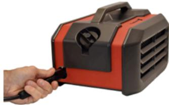
Attach the power cord from the power brick to the back of the machine until a “click” is heard.
